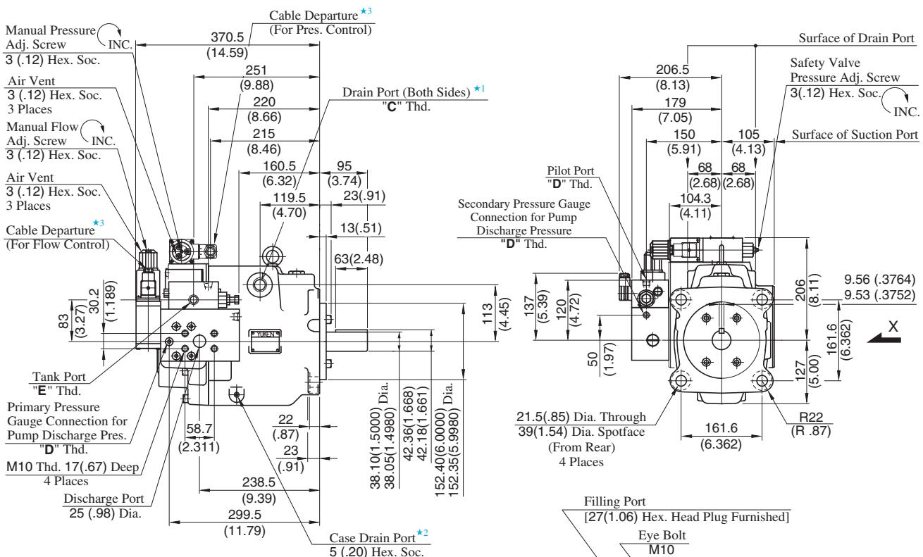
★ 1. Use either port of two drain ports at your option. Keep the remaining port plugged.
