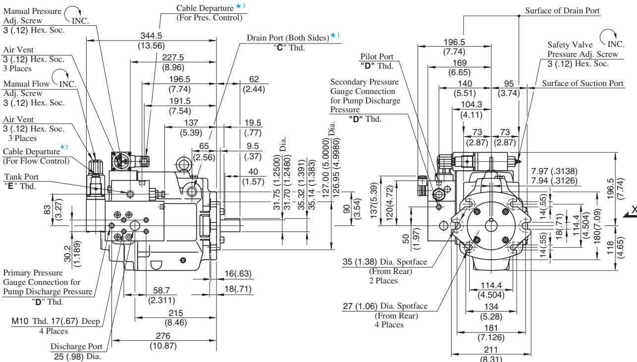
★ 1. Use either port of two drain ports at your option. Keep the remaining port plugged.
