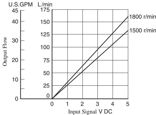
Note: Pump characteristics at 1800 r/min is the same as those at 1500 r/min where frequency is compensated.
