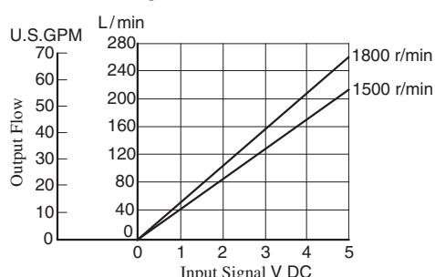
Note: Pump characteristics at 1800 r/min is the same as those at 1500 r/min where frequency is compensated.
