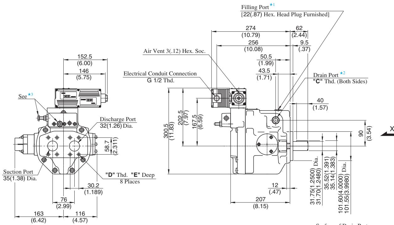
★1. Install the pump so that the "Filling Port" is at the top.
