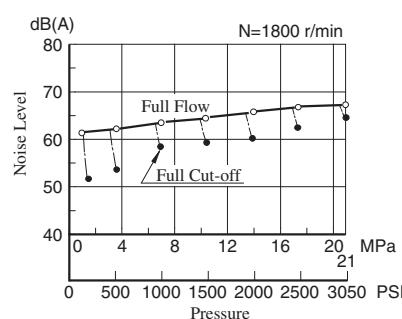
Typical Performance Characteristics of Type "A56" at Viscosity 20 mm<sup>2</sup>/s (100 SSU) [ISO VG32 Oils, 50°C (122°F)]
