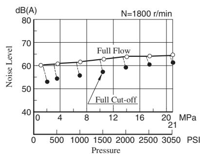
Typical Performance Characteristics of Type "A22" at Viscosity 20 mm<sup>2</sup>/s (100 SSU) [ISO VG32 Oils, 50°C (122°F)]
