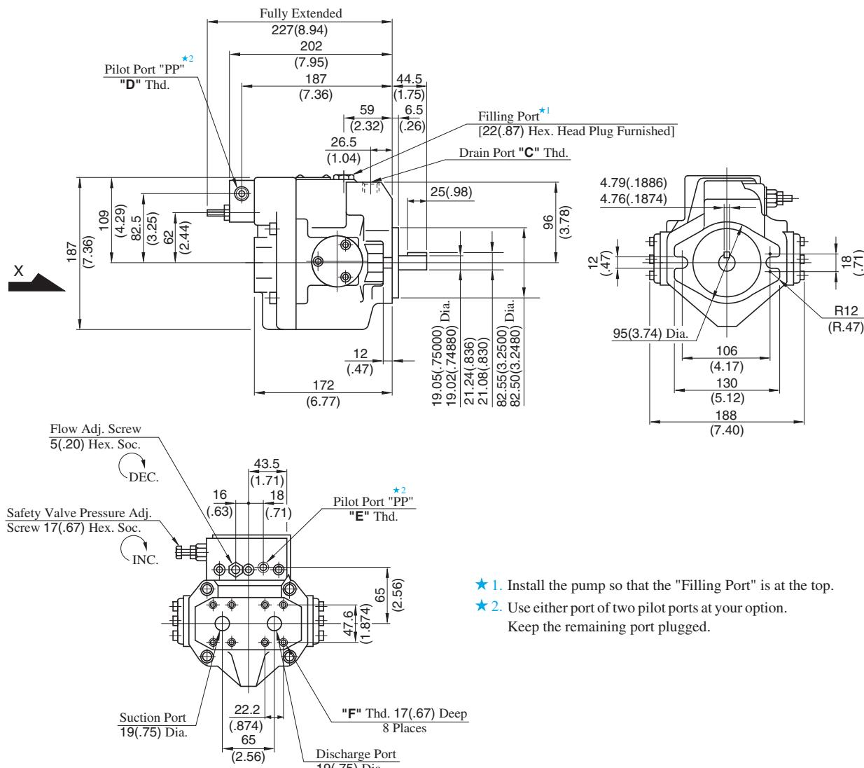
★ 1. Install the pump so that the "Filling Port" is at the top.
