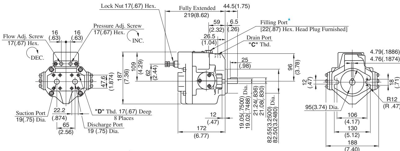
★ Install the pump so that the "Filling Port" is at the top.
