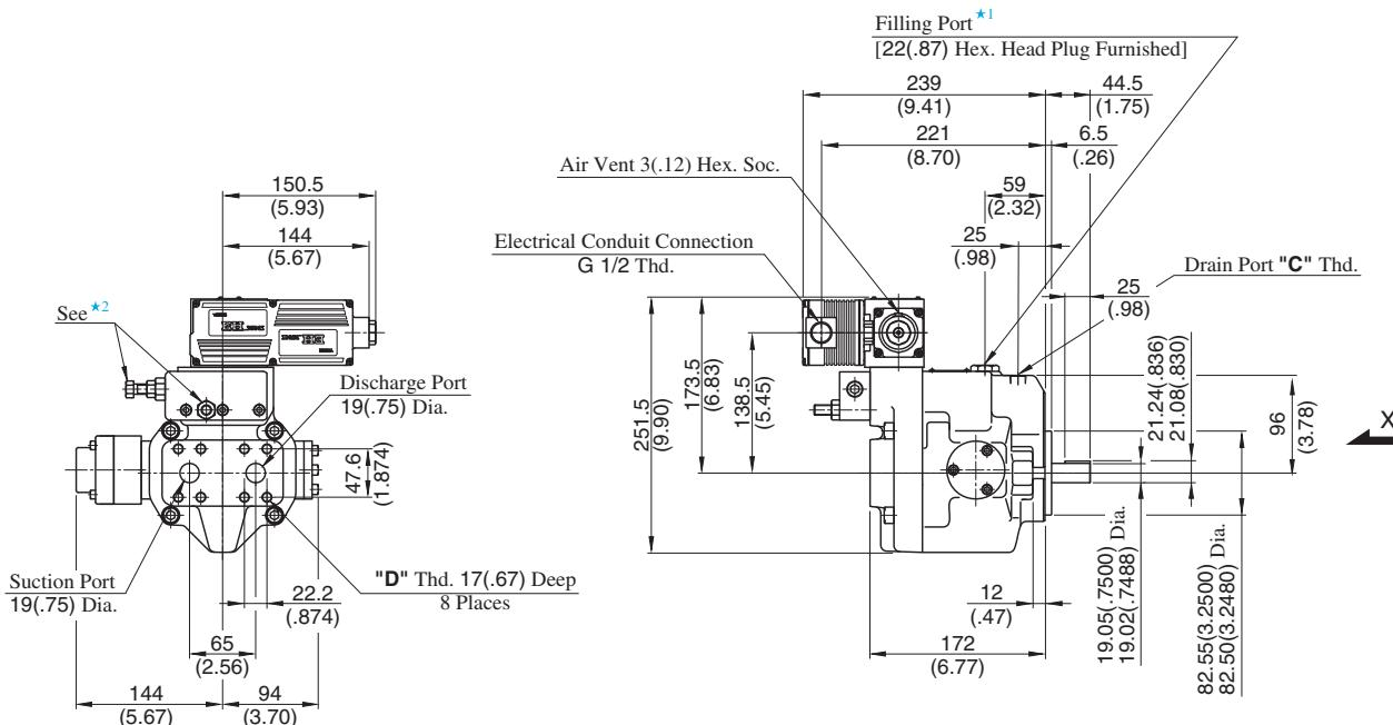
★1. Install the pump so that the "Filling Port" is at the top.
