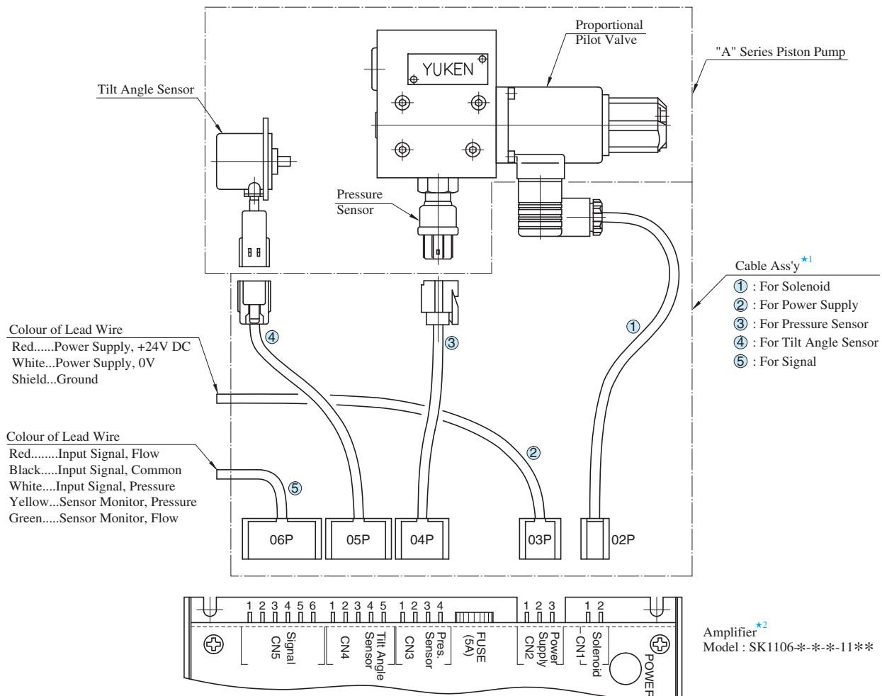
★1. Cable assemblies are available. When ordering, specify the cable ass'y model numbers from the table below.
