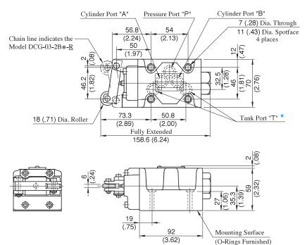
★. Although the tank port is shown on the left in our sub-plate, either may be used.
